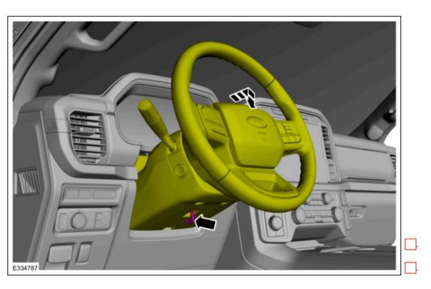
7. Release the tabs and disconnect the gap hider from the upper steering column shroud. Remove the General Equipment: Interior Trim Remover
