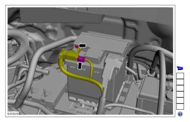
4. NOTICE: Make sure the battery cable terminal is properly positioned to the battery monitoring sensor before tightening the nut or component damage may occur.
