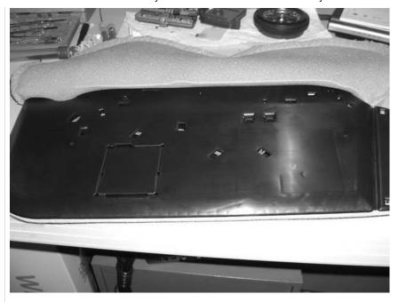
In this picture, the entire cloth was removed, but it's not nessesary. Just pull back enough to cut out the plug and do the wiring (either to a lighted mirror (if equipped), or extend the wiring out of the visor.
