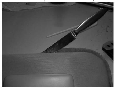
This picture shows how to use a simple butter knife to carefully seperate and remove the cloth cover. You don't have to remove all the cloth; just about half of the upper corner to gain access to the part in the hard plastic that will be removed to snap the **Homelink** module into.
