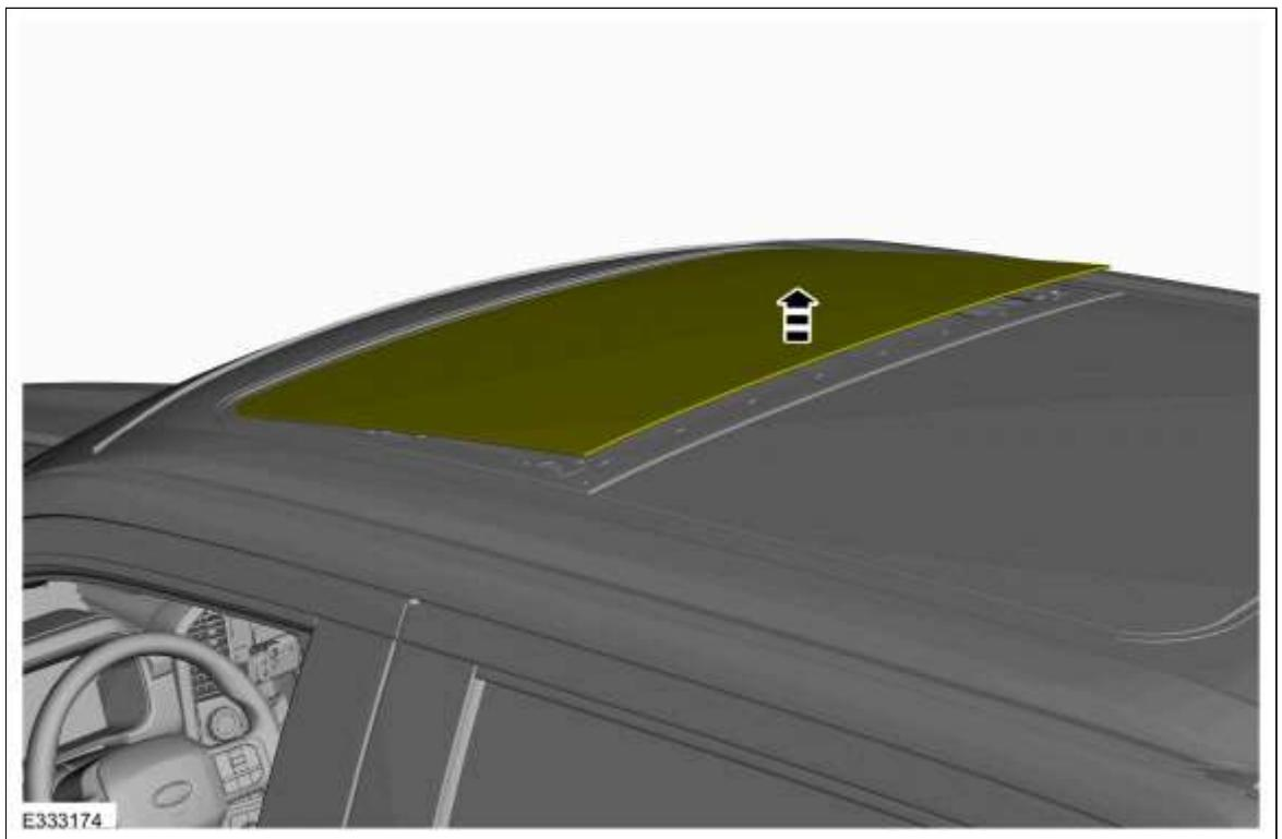
2. **NOTE:** During installation, make sure the blind is fully seated. An audible noise will be heard when the blind seats to the lower bracket.
